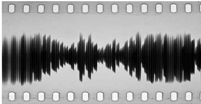
Berglund optical sound negative on nitrate film, c.1922. Multiple optical tracks across entire emulsion area. (Photo: Mark Standley)
